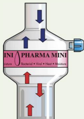
Heat and moisture passing through the HME filter
